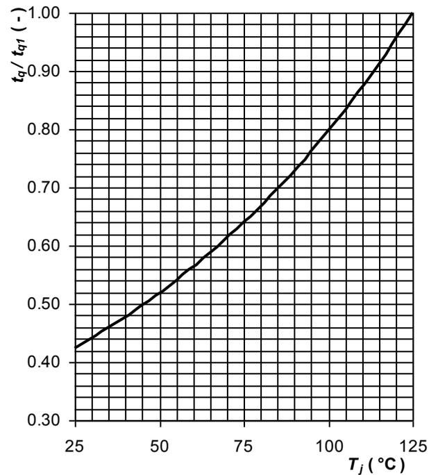
Fig. 12 Normalised maximum turn-off time vs. junction temperature
